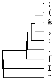
FIGURE 5.19: One of several classes of punctuation characters discovered from the Sherlock corpus at the character level by the agglomeration algorithm.
