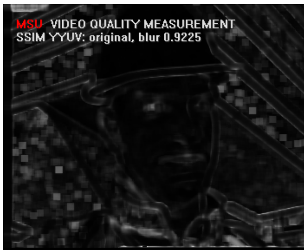
(c) SSIM map for blurred image, SSIM = 0.9225
