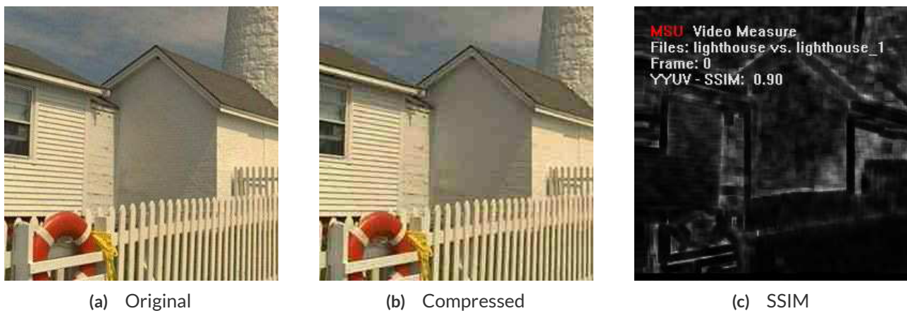
Figure 19: SSIM example for compressed image
