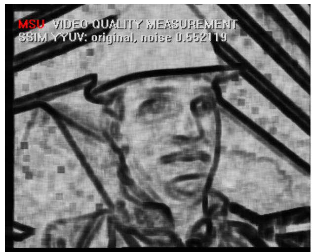
(b) SSIM map for noisy image, SSIM = 0.552119
