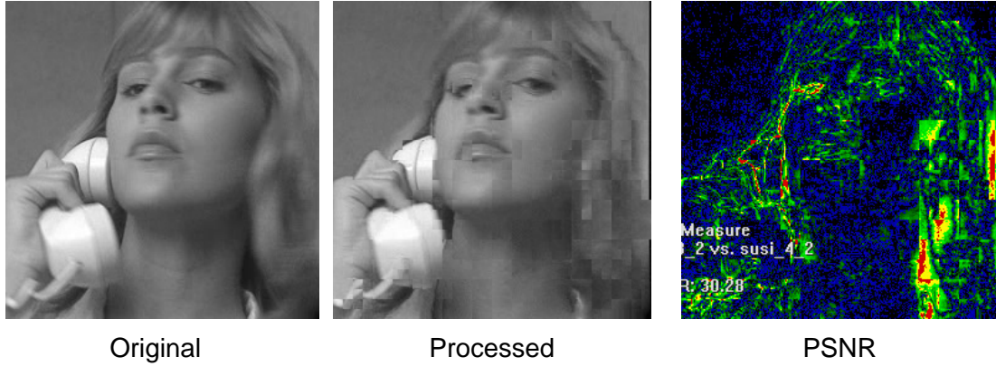
Figure 101. PSNR example for two frames
