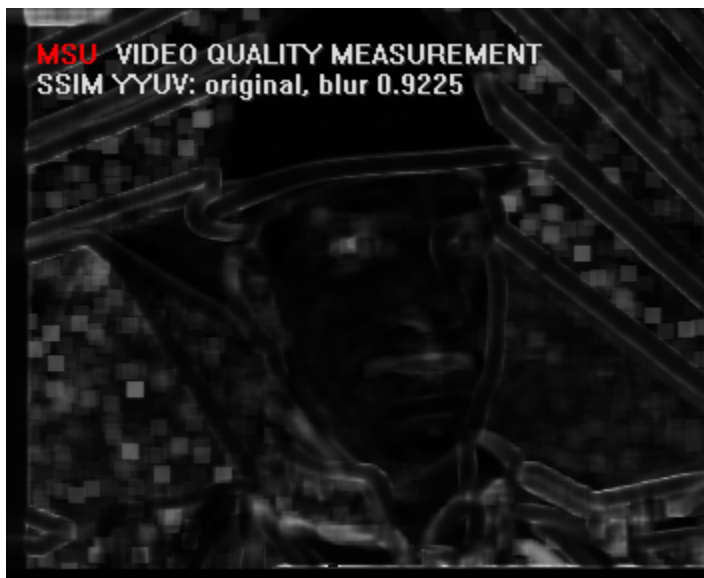
SSIM for image with blurred image, value = 0.9225
