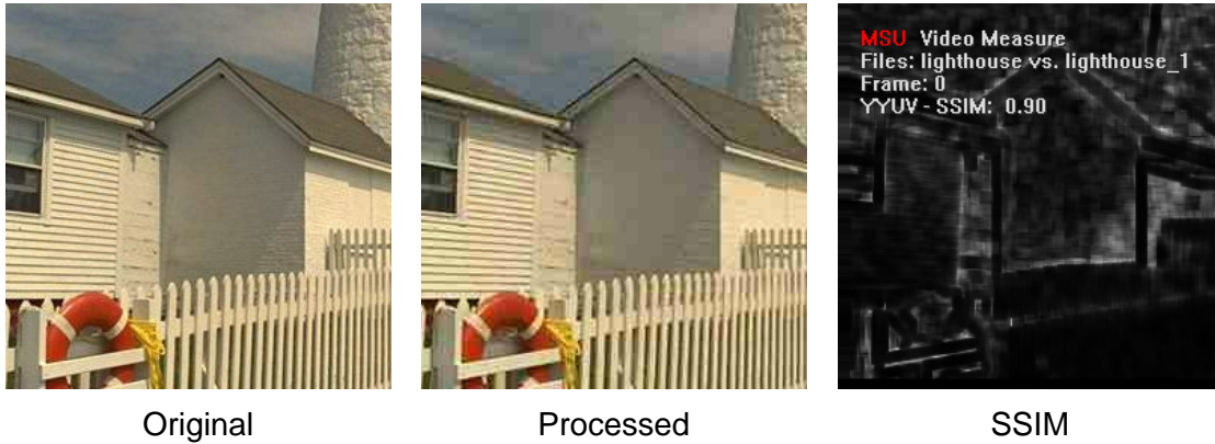
Figure 104. SSIM example for compressed image
