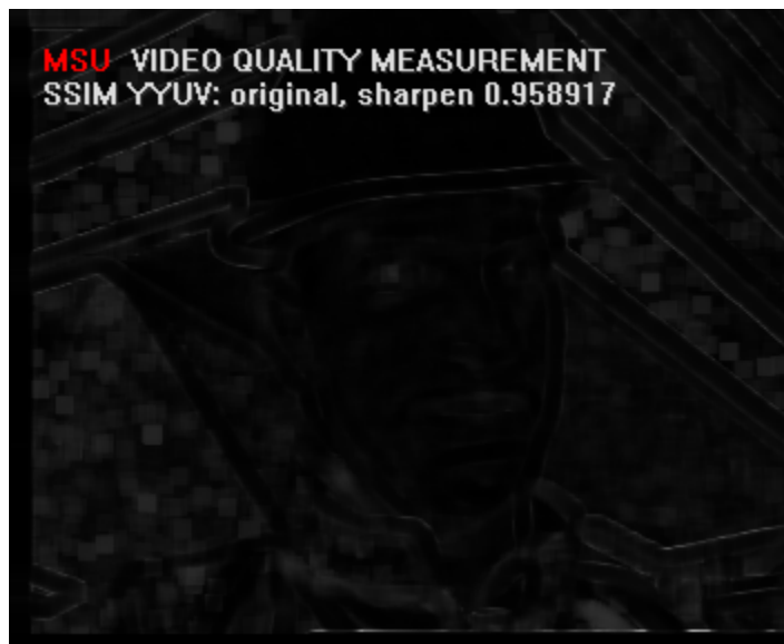
SSIM for image with sharpen image, value = 0.958917
