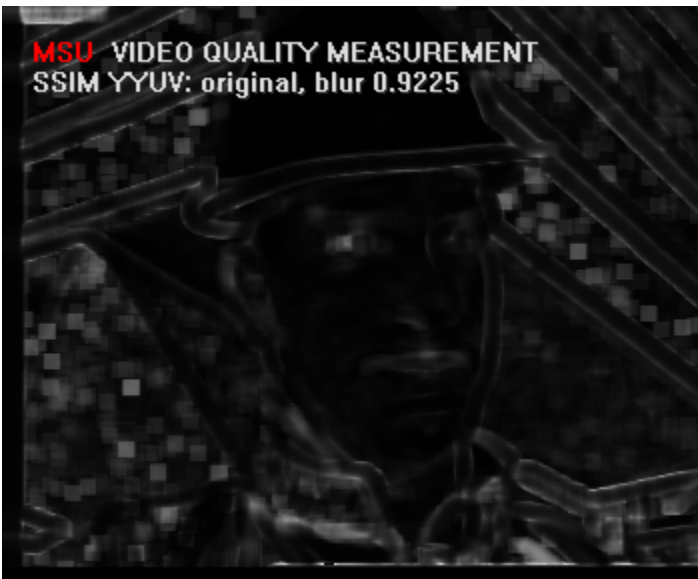
SSIM for image with blurred image, value = 0.9225
