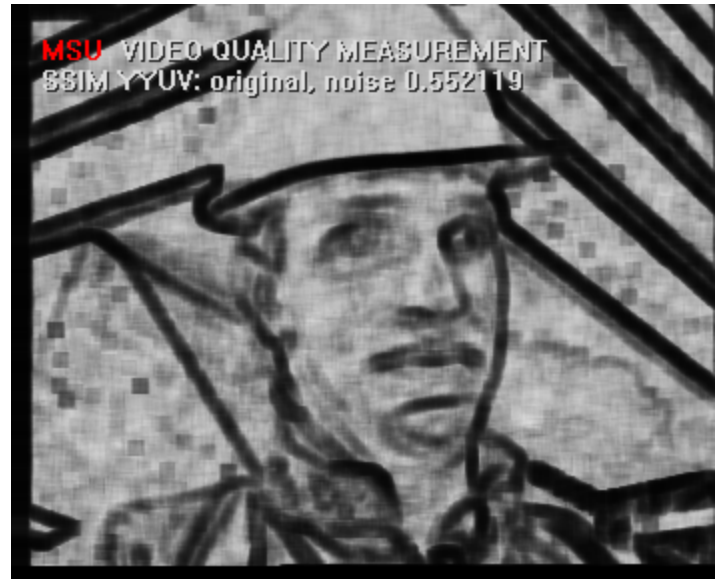
SSIM for image with noisy image, value = 0.552119
