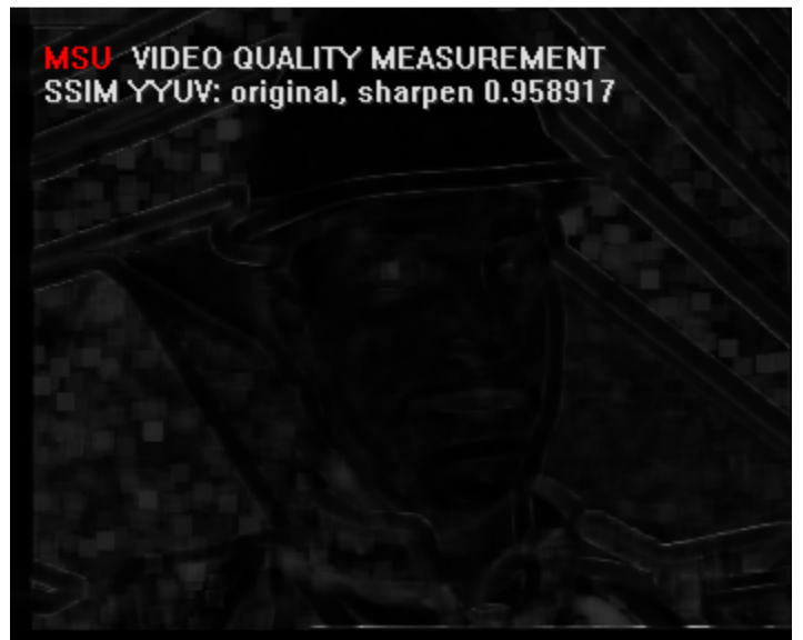
SSIM for image with sharpen image, value = 0.958917
