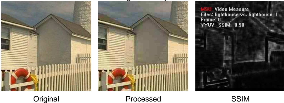
Figure 277. SSIM example for compressed image
