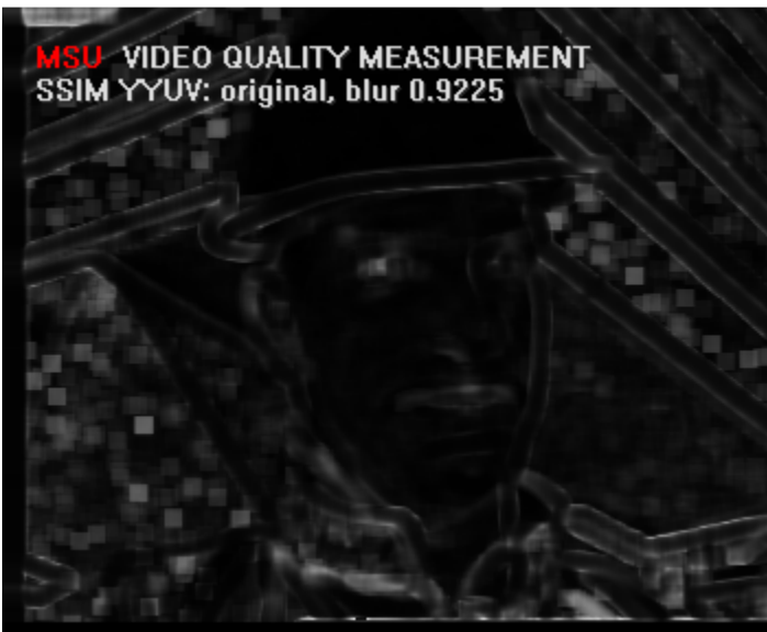
SSIM for image with blurred image, value = 0.9225
