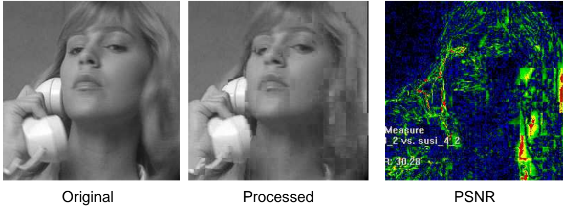
Figure 274. PSNR example for two frames
